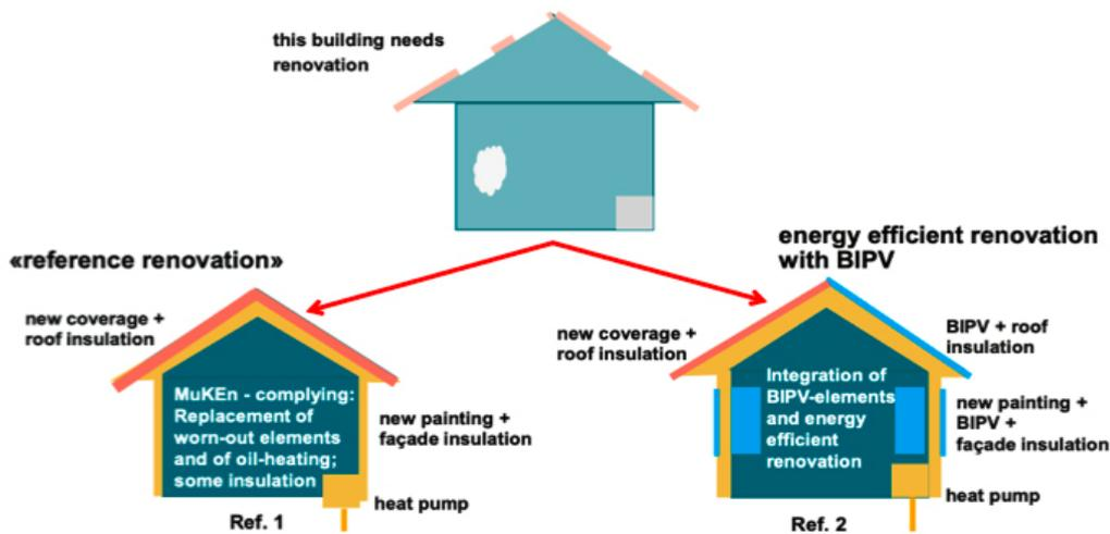
Fig. 1 Definition of a common "reference renovation" versus an energy efficient renovation with BIPV (©econcept).
