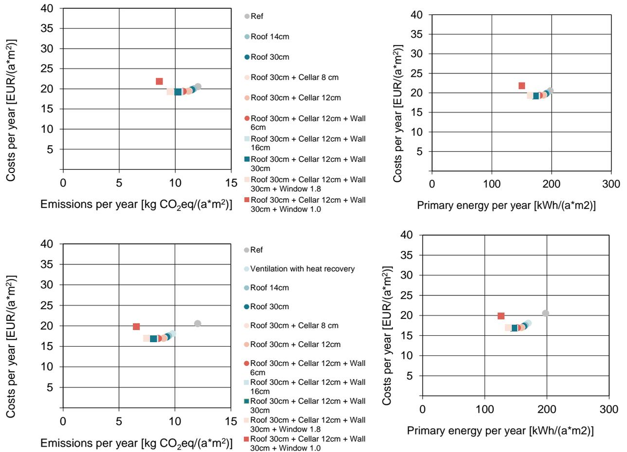
Figure 45 Effect of upgrading an existing ventilation system to a ventilation system with heat recovery on cost-effectiveness and environmental impacts of different renovation packages in a multi-family building in Sweden. The graphs above show renovation measures without improving the energy performance of the existing ventilation system; the graphs below show renovation packages with an upgrade of the ventilation system. The reference case is indicated with a grey dot.
