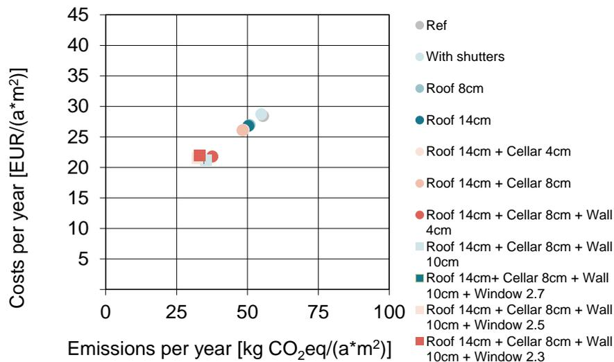
Figure 54 Comparison of emissions/cost curves for the generic building in Portugal without taking into account cooling (top) and with taking into account cooling (lower two figures). The latter case is differentiated in a situation without use of shutters (center), and with use of shutters (bottom).
