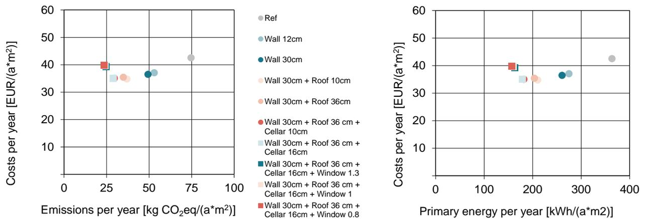
Figure 48 Comparison of calculations for a single-family building in Switzerland without including embodied energy (above) and with including embodied energy (below), for different renovation packages, including the renewal of an **oil heating system**. The reference case (grey dot) is virtually the same whether embodied energy is included or not, because embodied energy use of the activities in the reference case is so small.
