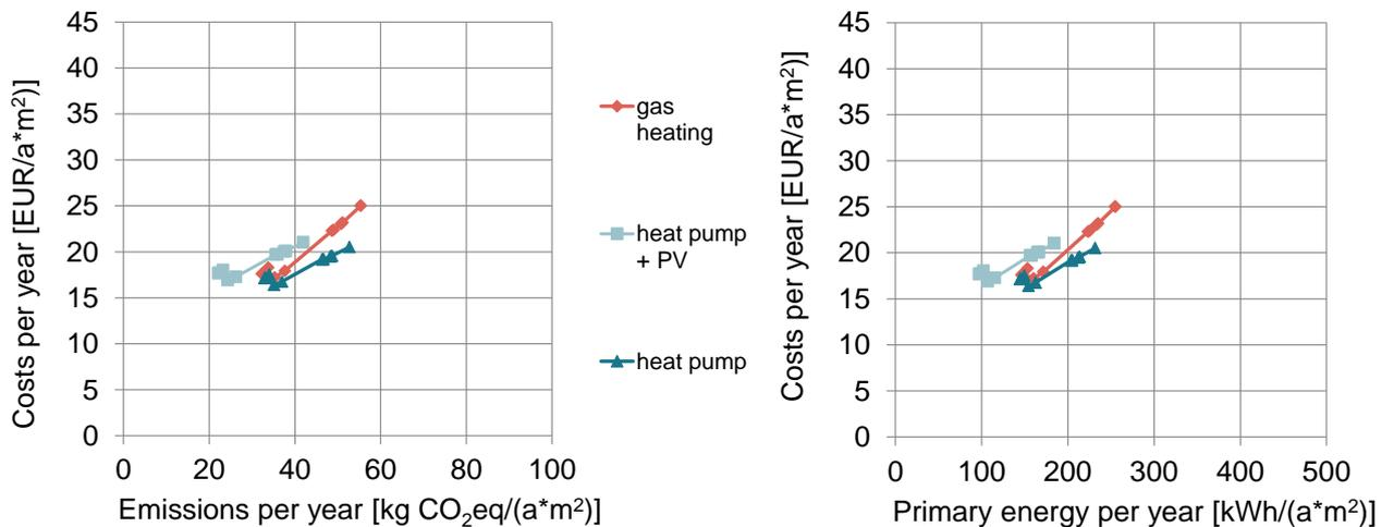
Figure 11 Aggregated comparison of cost-effectiveness of energy efficiency renovation measures for different heating systems and related impacts on carbon emissions and primary energy use in **Portugal**, for a **multi-family building**. The reference case is the point on the natural gas heating curve with the highest emissions/primary energy use, as no measures are carried out to improve the energy performance in that case.
