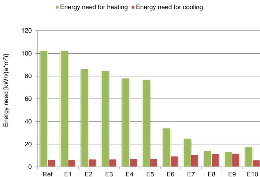
Figure 51 Energy need for heating and cooling for the generic multi-family reference building in Portugal.
