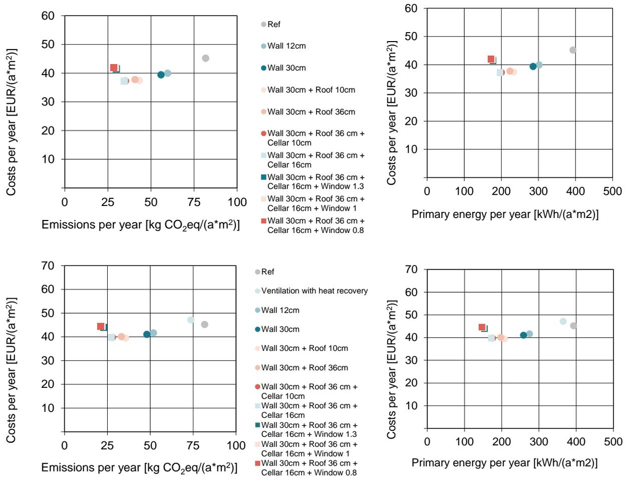
Figure 46 Effect of adding a ventilation system with heat recovery on cost-effectiveness and environmental impacts of different renovation packages in a single-family building in Switzerland, assuming an oil heating system. The graphs above show renovation measures without existing ventilation system; the graphs below show renovation packages with the inclusion of a ventilation system. The reference case is indicated with a grey dot. An oil heating system is assumed.
