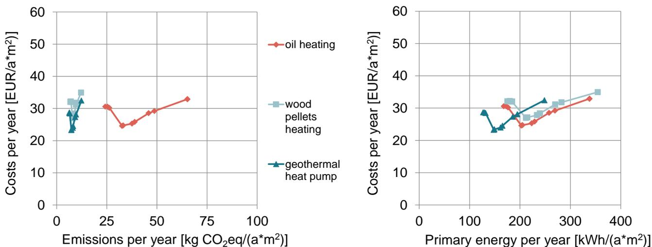
Figure 3 Aggregated comparison of cost-effectiveness of energy efficiency renovation measures for different heating systems and related impacts on carbon emissions and primary energy use in **Switzerland**, for a **multi-family building**. The reference case is the point on the oil heating curve with the highest emissions/primary energy use, as no measures are carried out to improve the energy performance in that case.
