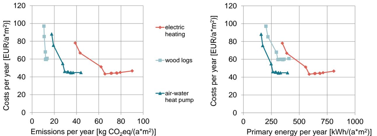
Figure 9 Aggregated comparison of cost-effectiveness of energy efficiency renovation measures for different heating systems and related impacts on carbon emissions and primary energy use in **Norway**, for a **single-family building**. The graphs are calculated with the residual electricity mix based on taking into account in addition also the import and export of guarantees of origin.
