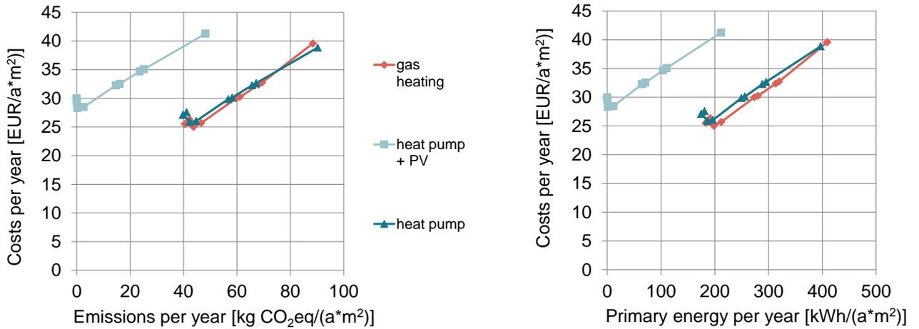
Figure 31 Aggregated comparison of cost-effectiveness of energy efficiency renovation measures for different heating systems and related impacts on carbon emissions and primary energy use in Portugal, for a single-family building. The reference case is the point on the natural gas heating curve with the highest emissions/primary energy use, as no measures are carried out to improve the energy performance in that case.
