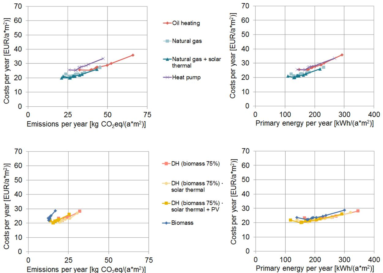
Figure 72: Aggregated comparison of cost-effectiveness of energy efficiency renovation measures for different heating systems and related impacts on carbon emissions and primary energy use for the Spanish case study
