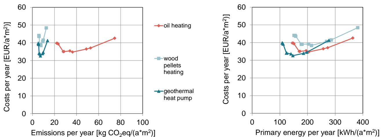
Figure 41 Aggregated comparison of cost-effectiveness of energy efficiency renovation measures for different heating systems and related impacts on carbon emissions and primary energy use in Switzerland, for a single-family building. The reference case is the point on the oil heating curve with the highest emissions/primary energy use, as no measures are carried out to improve the energy performance in that case.
