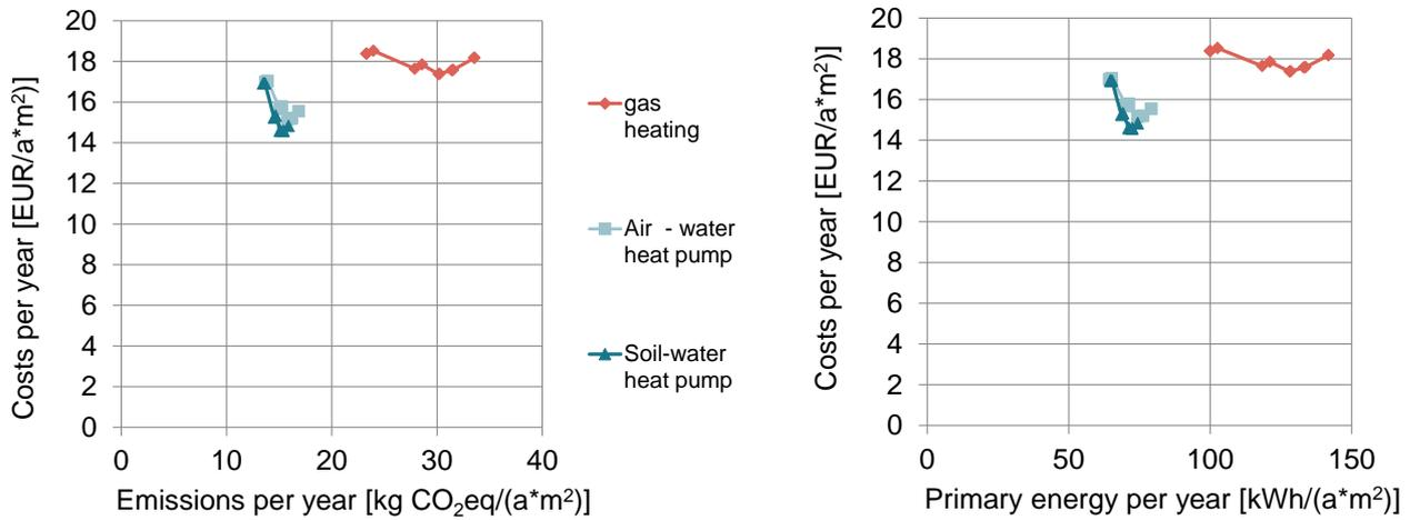
Figure 8 Aggregated comparison of cost-effectiveness of energy efficiency renovation measures for different heating systems and related impacts on carbon emissions and primary energy use in **Italy**, for a **multi-family building**. The reference case is the point on the gas heating curve with the highest emissions/primary energy use, as no measures are carried out to improve the energy performance in that case.
