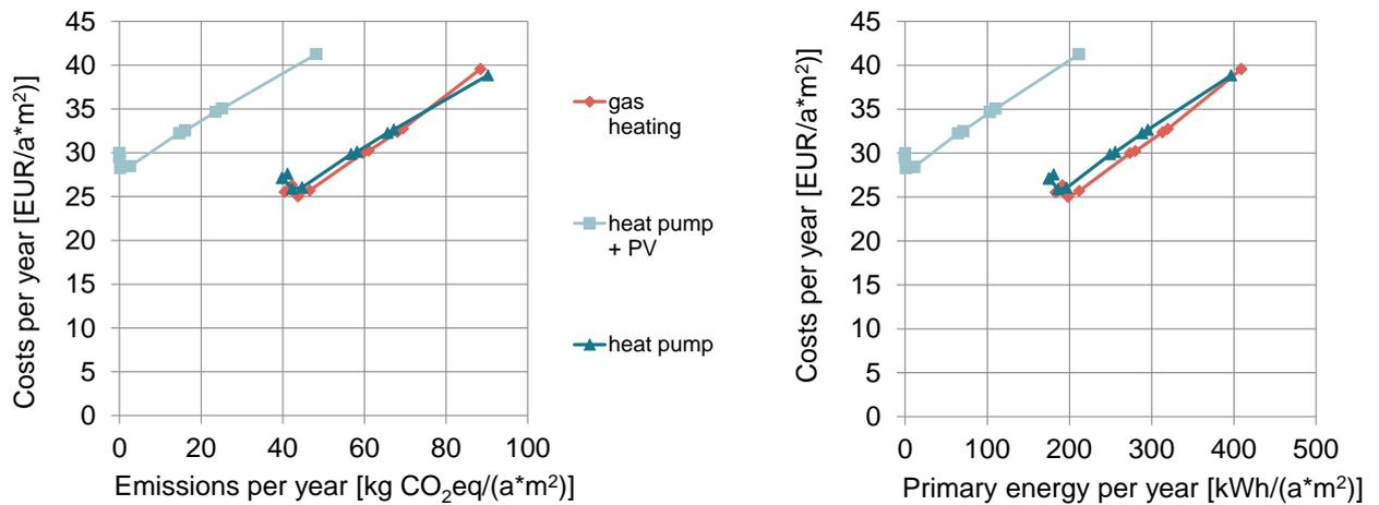
Figure 10 Aggregated comparison of cost-effectiveness of energy efficiency renovation measures for different heating systems and related impacts on carbon emissions and primary energy use in **Portugal**, for a **single-family building**. The reference case is the point on the natural gas heating curve with the highest emissions/primary energy use, as no measures are carried out to improve the energy performance in that case.
