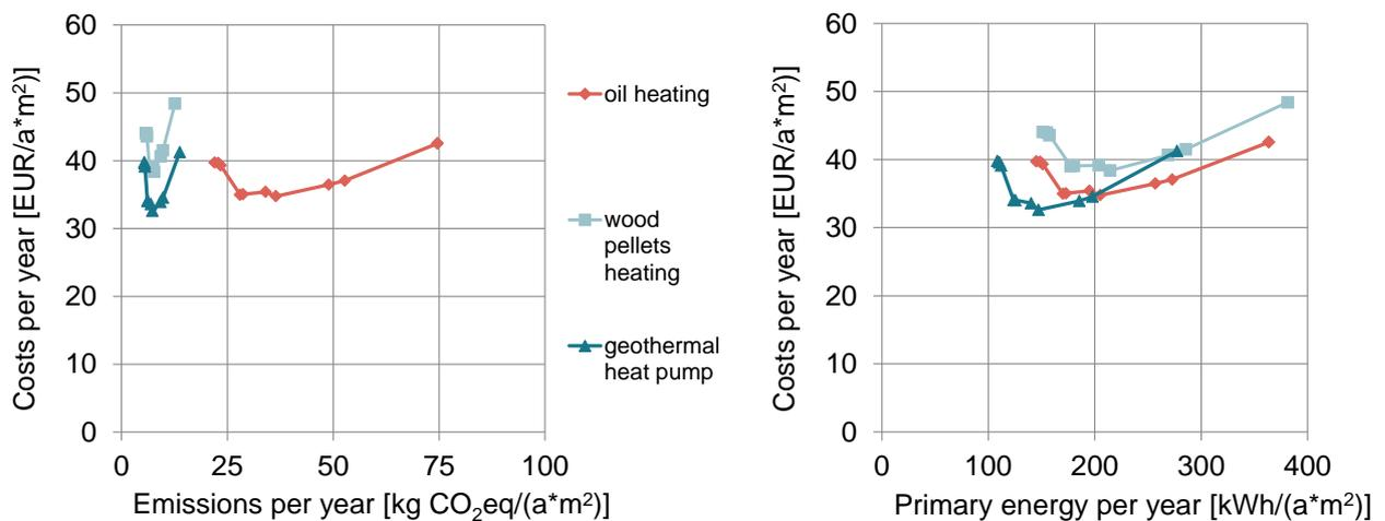
Figure 61 Aggregated comparison of different renovation packages for the single-family reference building in Switzerland
