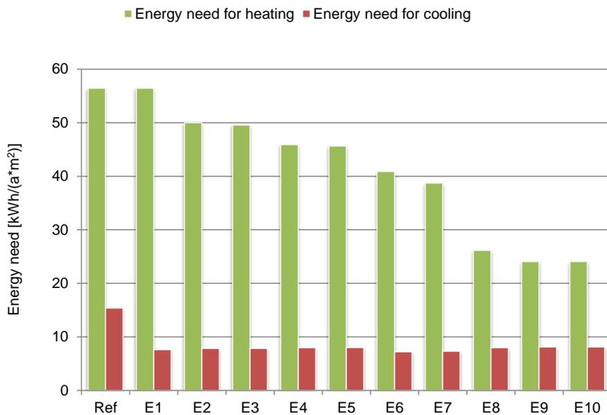
Figure 56 Energy need per year for heating and cooling for the generic reference building in Italy, taking into account the use of shutters.
