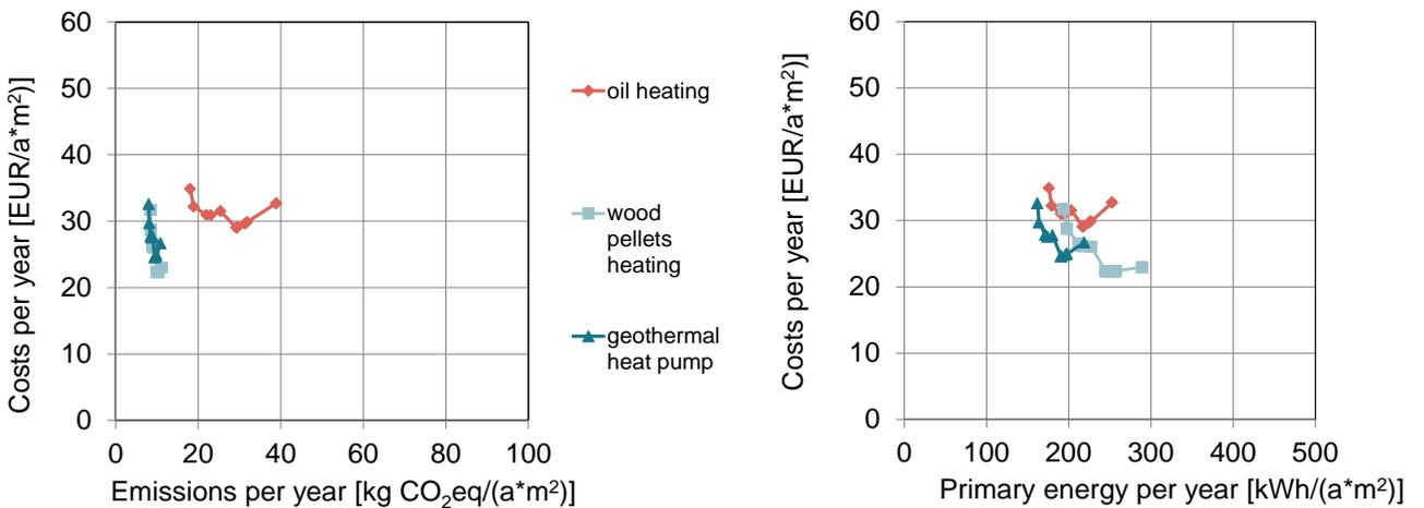
Figure 7 Aggregated comparison of cost-effectiveness of energy efficiency renovation measures for different heating systems and related impacts on carbon emissions and primary energy use in **Denmark**, for a **multi-family building**. The reference case is the point on the oil heating curve with the highest emissions/primary energy use, as no measures are carried out to improve the energy performance in that case.
