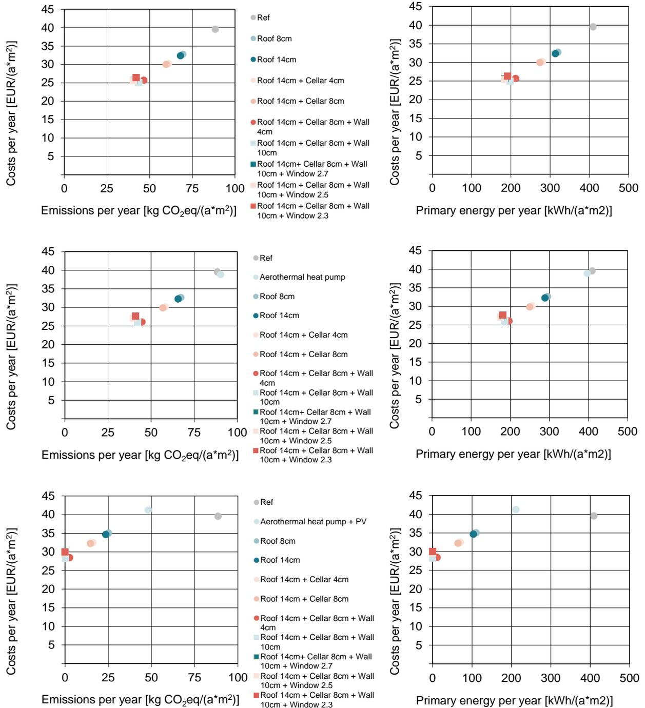
Figure 30 Comparison of cost-effectiveness of energy efficiency renovation measures for a single-family building in Portugal for different heating systems, gas (top graphs), air-water heat pump (middle) and air-water heat pump + PV (bottom), as well as related impacts on carbon emissions and primary energy use. In all graphs, the reference shown as a grey dot refers to a
