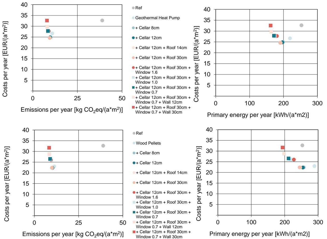
Figure 23 Aggregated comparison of cost-effectiveness of energy efficiency renovation measures for multi-family building in Denmark for different heating systems, oil (top graphs), geothermal heat pump (middle), wood pellets (bottom), and related impacts on carbon emissions and primary energy use. The reference case is the point on the oil heating curve with the highest emissions/primary energy use, as no measures are carried out to improve the energy performance in that case.
