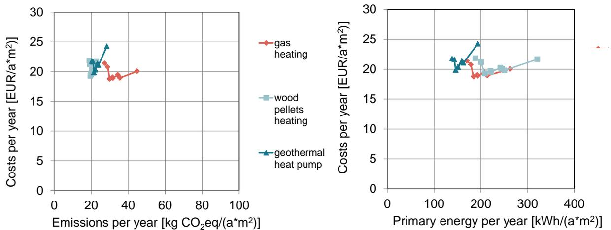
Figure 35 Aggregated comparison of cost-effectiveness of energy efficiency renovation measures for different heating systems and related impacts on carbon emissions and primary energy use in Spain, for a multi-family building. The reference case is the point on the natural gas heating curve with the highest emissions/primary energy use, as no measures are carried out to improve the energy performance in that case.
