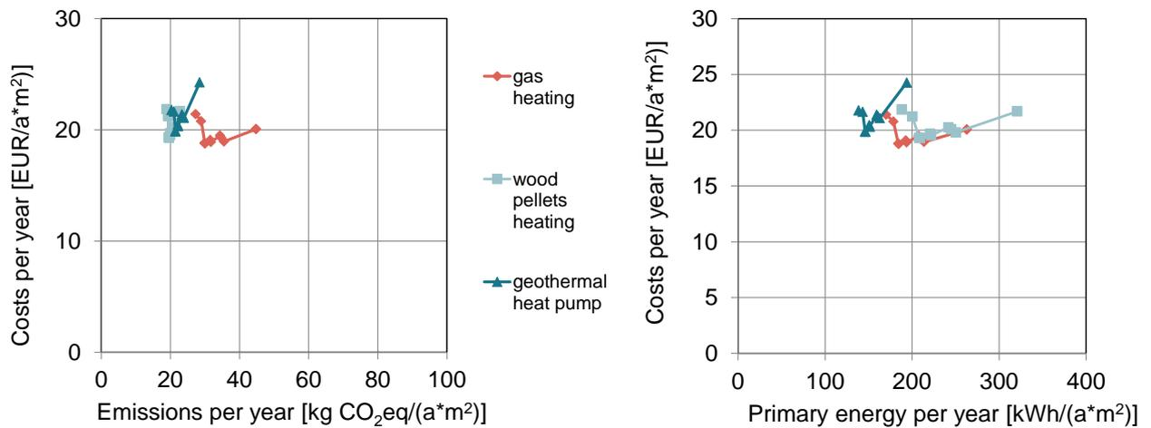
Figure 12 Aggregated comparison of cost-effectiveness of energy efficiency renovation measures for different heating systems and related impacts on carbon emissions and primary energy use in **Spain**, for a **multi-family building**. The reference case is the point on the natural gas heating curve with the highest emissions/primary energy use, as no measures are carried out to improve the energy performance in that case.
