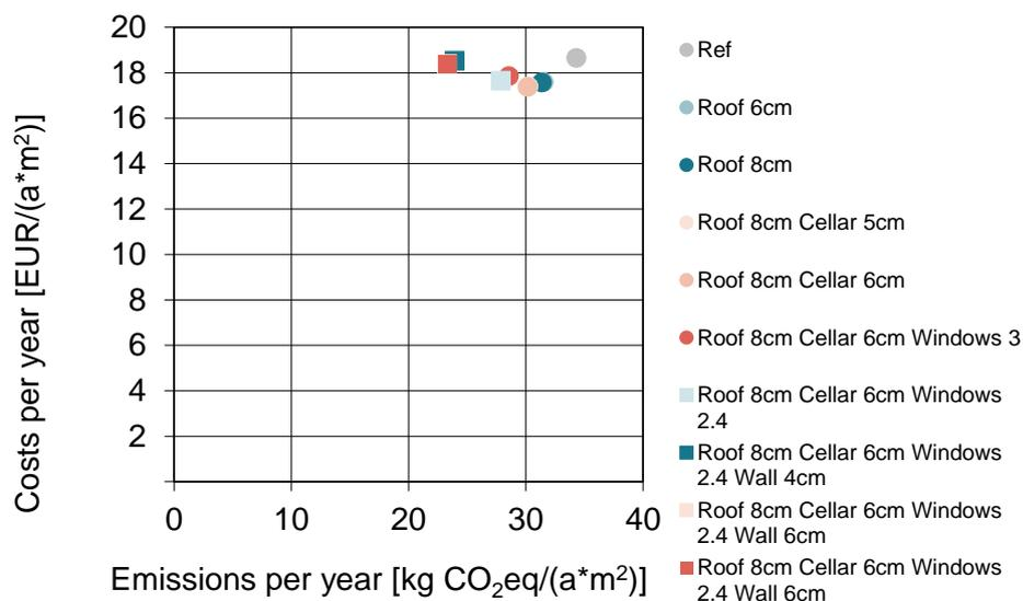
Figure 57 Comparison of emissions/cost curves for the generic building in Italy without taking into account cooling (top) and with taking into account cooling (lower figure). When cooling is taken into account, the use of shutters is assumed. For the related calculations, no costs have been taken into account for the shutters or the cooling system; it is assumed they are already part of the building.
