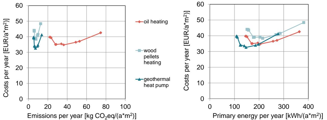
Figure 15 Aggregated comparison of cost-effectiveness of energy efficiency renovation measures for different heating systems and related impacts on carbon emissions and primary energy use in **Switzerland**, for a **single-family building**. The reference case is the point on the oil heating curve with the highest emissions/primary energy use, as no measures are carried out to improve the energy performance in that case.
